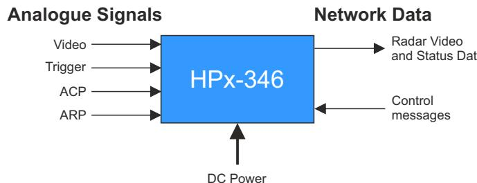
With the HPx-346 unit, an analogue radar video output can quickly and easily be turned into an open network data stream that multiple clients can access.
