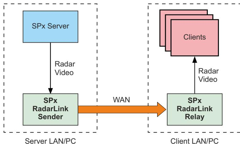
SPx RadarLink addresses the problems of unreliable or low data rate connections using three approaches:
