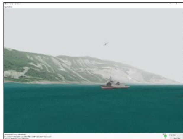
Given a lat/long location for the camera (whether moving or static), SPx Video Simulator generates a real-time image of the view that the camera can see from that location. This incorporates terrain that is visible from that location, as well as any targets. In the above example, a moving drone is visible in the first image and a ship in the second. The video image is correctly updated in real-time to reflect the motion of the targets in the world and the motion of the camera platform itself.
