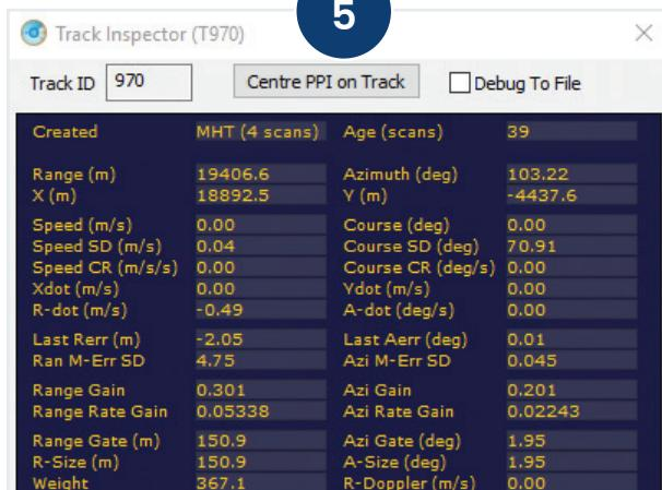
Track inspector provides detailed information about a selected radar track, including details of the tracking gate.
