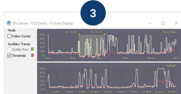
Graphical tools, such as an A-scan display, are available to assist with process configuration.
