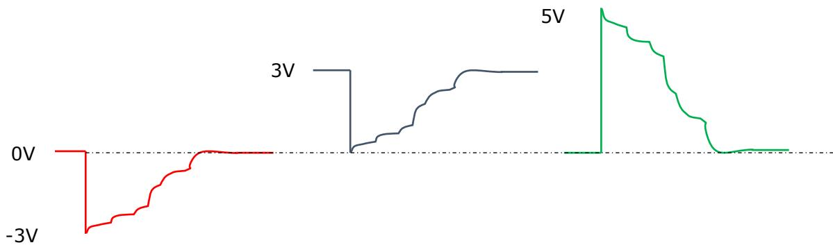
1. The video signal coming from the radar ranges from 0V (no signal / black level) to -3V peak.
