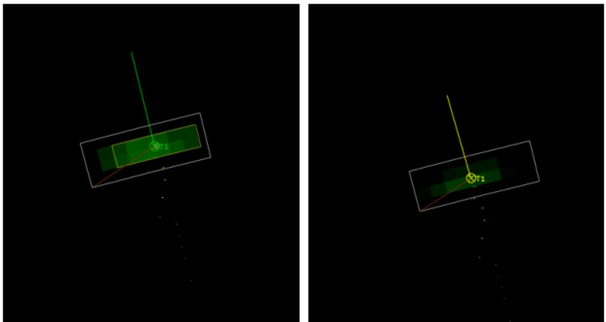
One application of TfV is to extend the time of tracking of a target by permitting updates after plots are lost. However, the success of this depends on there being some low-level, intermittent target video present. If there is no video present then TfV will have no affect and the track will coast as normal. In this situation there is nothing lost by enabling TfV.
